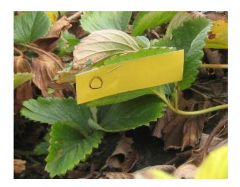
Figure 2. Water sensitive paper stapled to outer leaf of strawberry plant
